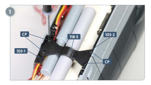
Position the crossmember **118-5** over the silencer and the upper torpedo housing (see inset photograph). Attach it to the connectors **103-1** and **103-2** using two **CP** screws at each end. Take care not to overtighten the screws.
