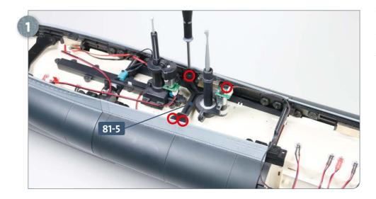
The final task is to remove the previously installed connector **81-8** and replace it with a slightly different one: this will remove a small gap in the port (L) side of the hull. First, remove the four **CP** screws (locations circled in red) that hold the crossmember **81-5** in place.
