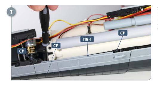
Join the hull section **118-1** to the main structure using three **CP** screws, one each onto connectors **99-2**, **99-4** and **103-2**. Note that one of the **CP** screws cannot be seen and is located at the bottom end of the screwdriver.
