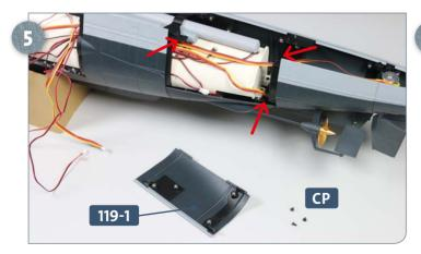
Position the hull section **119-1** next to the main structure, as shown, and have ready three **CP** screws. The three arrows indicate the points (connectors) to which the plate is attached to the hull.
