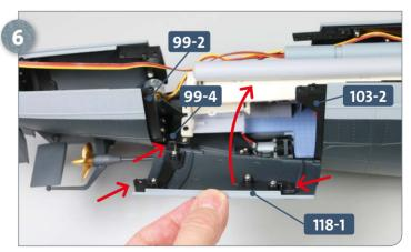
Position the hull section **118-1** on the starboard (R) side of your model. The holes of the connectors (indicated by the three straight arrows) align with the holes in connectors **99-2**, **99-4** and **103-2**.
