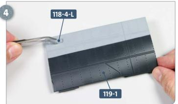
Apply a little glue to the peg on the inside of the port exhaust **118-4-L**. Fit the exhaust in the slot in the hull section **119-1**, oriented as shown in the photo above.
