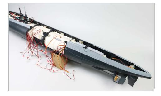
Another hull section has now been added to the port (L) side of the model. In addition, a crossmember has been fitted and one of the previously fitted connectors has been replaced with a new one.
