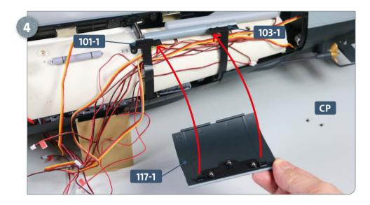
Place the model on your worktop so that you have access to the port (L) side. Have ready two **CP** screws. Placing the lip of the hull section **117-1** on the edge of the keel at the aft end of the sixth compartment, tilt the hull plate upwards towards the two connectors, **101-1** and **103-1**, as indicated by the arrows, left.
