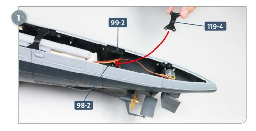
Take the crossmember **119-4** and align its holes over the corresponding holes in connectors **98-2** and **99-2**, as shown.
