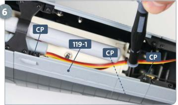
Making sure that no wires have become trapped, fix the hull plate **119-1** in place using three **CP** screws, as pictured.
