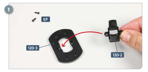
Place the lower rear bracket **120-3** and two **EP** screws on your work surface. Take connector **120-2** and fit the two screw tabs at the sides into the recesses of the bracket, as indicated by the arrow.
