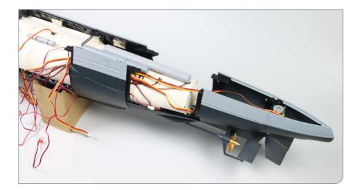
A new hull plate has now been added to the port (L) side of the hull.
