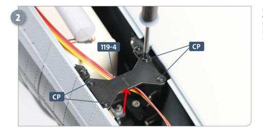
Make sure that the arrow embossed in the centre of the crossmember **119-4** (indicated by the red arrow) points towards the bow. Fix in place to the aforementioned connectors using two **CP** screws on each side.
