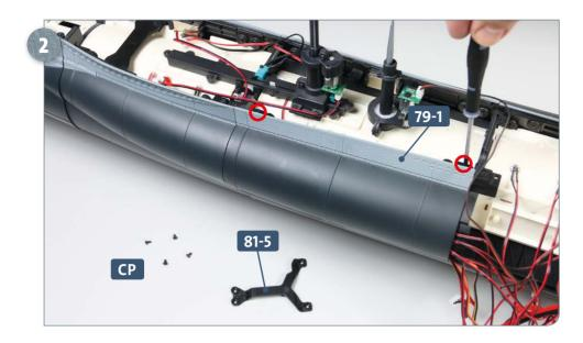
Place the four **CP** screws safely to one side and remove the crossmember **81-5** as shown. Now, turn to the port (L) hull section **79-1** and remove the two **CP** screws attaching it to the main hull structure (circled in red).
