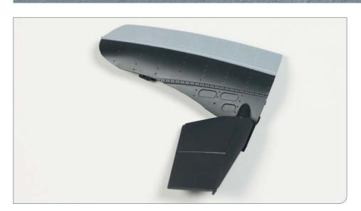
Two connectors and the starboard (R) rudder have now been attached to the starboard (R) tail section.
