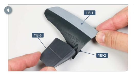
Take the starboard (R) rudder 113-5 and guide its shaft through the hole in the tail section 113-1 and into the connector behind it 113-2.
