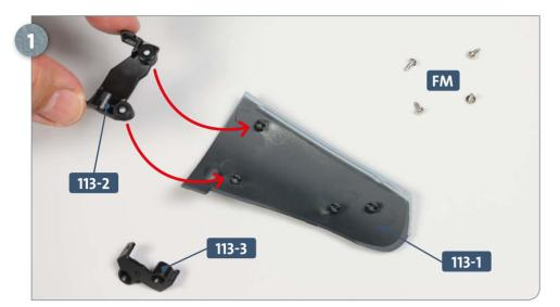
Place the starboard (R) tail section 113-1, both connectors 113-2 and 113-3 and four FM screws on your work surface. Take connector 113-2 and fit it onto the two raised sockets at the forward end of the tail section, as indicated. Pay attention to the correct orientation of the connector.
