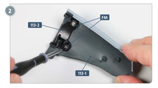
Fix the connector 113-2 in place with two FM screws.
