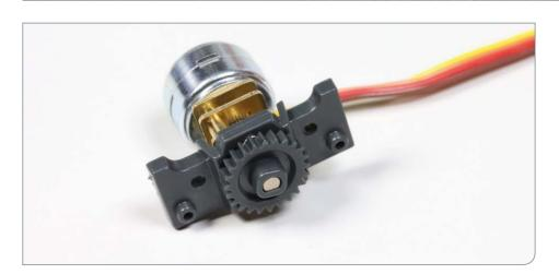
The motor for the rudder has now been fitted with a mounting plate and a cog.
