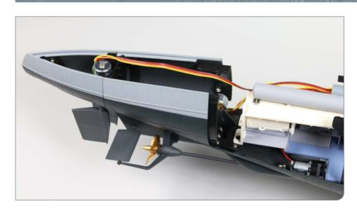
Both tail sections have now been attached to the hull, the stern torpedo tube is mounted, and the rudder motor has been installed.
