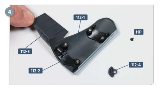
Have ready the swivel gear 112-4 and one HP screw. Take the port (L) rudder 112-5 and guide its shaft through the hole in the tail section 112-1 and into the connector 112-2, as shown in the photo.
