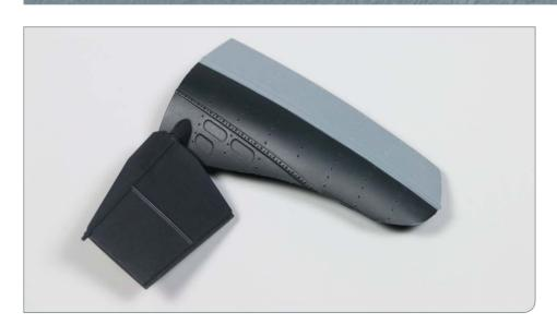
Two connectors and the port (L) rudder have now been attached to the port (L) tail section.
