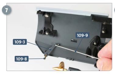
Fit the large hole at the other end of the lever 109-3 over the free end of the shaft 109-8. Pay attention to the alignment of both the lever 109-3 and the control rod 109-9.
