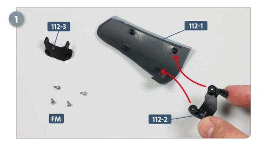
Place the port (L) tail section 112-1, both connectors 112-2 and 112-3 and four FM screws on your work surface. Take connector 112-2 and fit it onto the two raised sockets at the forward end of the tail section, as indicated. Pay attention to the correct orientation of the connector.
