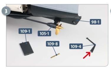
Working from the outside of hull plate 98-1, have ready the port (L) diving plane 109-1, the port (L) deflector rod 109-4, (identifiable by the notch, see arrow), and the shaft 109-8.
