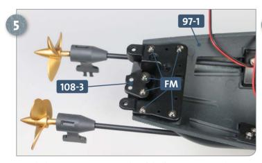
Attach the connector **108-3** to the aft hull section **97-1** with six **FM** screws, as pictured. In the next step, the electric motor room is inserted into the main structure.
