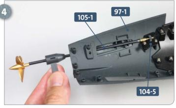
Guide the shaft of the propeller assembly **105-1** through the rectangular opening in the port (L) side of the aft hull section **97-1**. The cog at the forward end of the shaft fits into the recess in the motor housing **104-5**, as shown.
